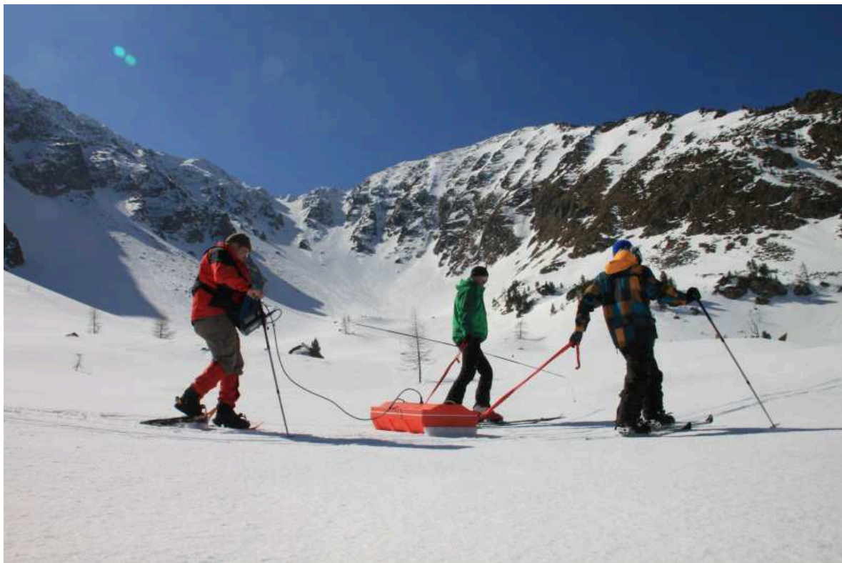
Fig. 8: Field impression of the ground-penetrating radar measurements on the Schöneben Rock Glacier in March 2012 (photo by courtesy of A. Kellerer-Pirklbauer)
